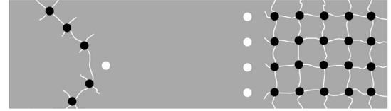
**Removing the top layer of a thicker rock massif** begins with drilling a few shallower holes to remove the toe and obtain a regular, vertical free surface of the cliff. Then more holes parallel to the new cliff surface, and reaching a few centimetres below the desired cut-off level, are drilled. One (best) or two consecutive rows are then filled up every 5 to 15 hours.
